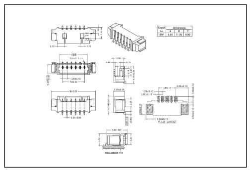
Figure 6: ACM1552U-Y USB Connector (Male) Specification
