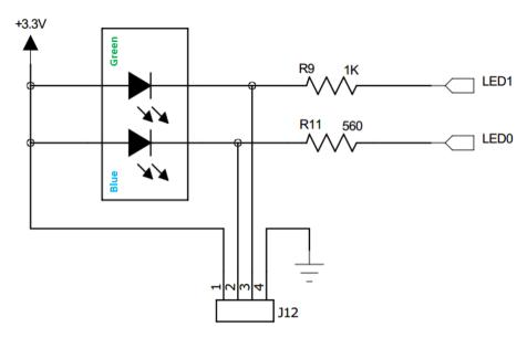
Figure 4: ACM1552U-Y LED Circuit
