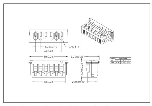
Figure 7: ACM1552U-Y Cable Connector (Female) Specification
