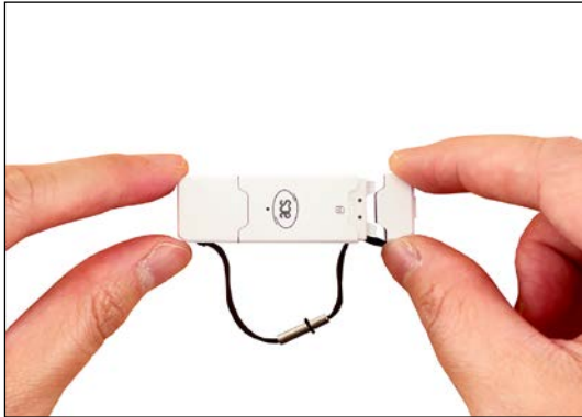
1. Remove the cap at the rear end of the reader.
