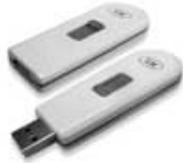
The ACR122T is designed with mobile applications in mind. Its compact, highly portable and extractable USB plug design make it easy to use, and suitable for integration into fast-paced environments. It is ideal for a wide range of NFC applications, such as secure computer log-on with corresponding contactless cards or NFC tags in public places like a coffee shop or public library, balance-checking and reloading of an e-Purse, and online payment.
